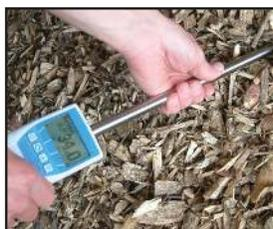
The BLL employs a 39" (one meter) long insertion probe that makes it easy to measure moisture content in deep piles of wood chips quickly and accurately. The process takes seconds and requires no prior sample preparation.
